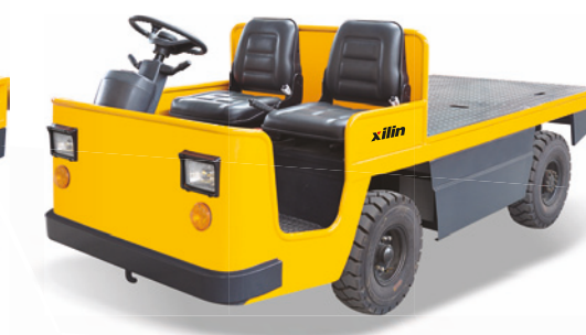
Electric platform tractor Model: BD20/BD25/BD30 Cap. : 2000kg, 2500kg, 3000kg
