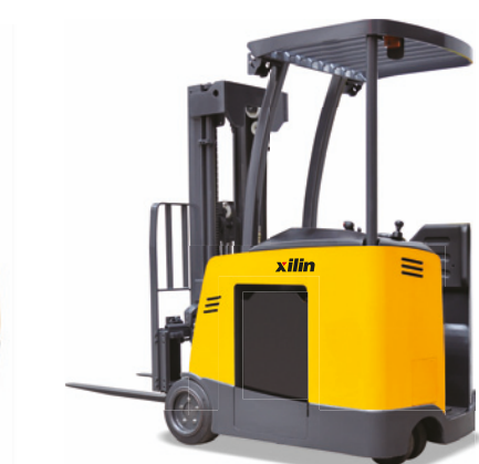
Stand-up Counterbalance Forklift Model: CPD20SR-16/CPD20SR-18 Cap. : 1600kg, 1800kg Lift height: 4.8m~6m
