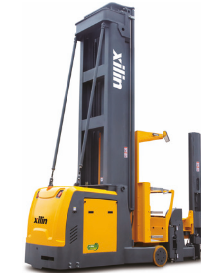
VNA Swing Reach Truck (man-up) Model: OPT15 Cap. : 1500kg Lift height: 5m~14.5m
