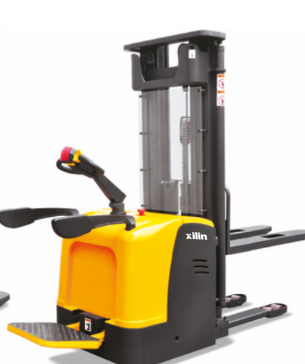
Electric stacker Model: CDDK15-I/CDDK15-II/CDDK15-III/CDDK20 Cap. : 1500kg, 2000kg Lift height: 2.5m~6.5m
