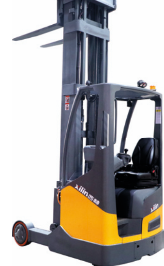
Electric reach truck Model: CQD16-LI Cap. : 1600kg Lift height: 5~11.1m
