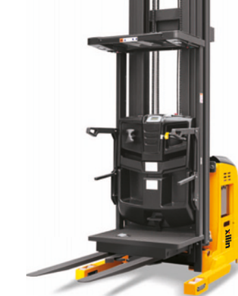
Electric high level order picker Model: OPS15 Cap. : 1500kg Lift height: 5m~11m
