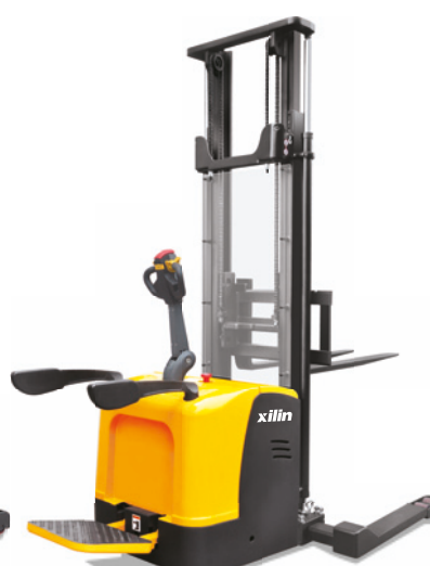
Electric straddle stacker Model: CTD15-I/CTDK15-II/CTDK15-III Cap. : 1500kg Lift height: 2.5m~5.6m
