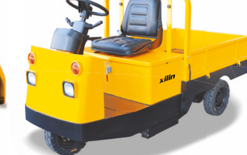
Electric platform tractor Model: BD10SE/BD20SE Cap. : 1000kg, 2000kg
