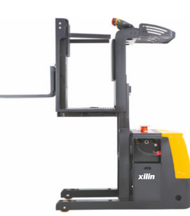
Middle level order picker Model: OPL10S/OPL12G Cap. : 1000kg, 2000kg Lift height: 1m~1.2m
