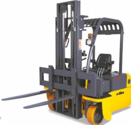
4-Directional Forklift Model: CSD16/CSD20 Cap. : 1600kg, 2000kg Lift height: 3m~6m
